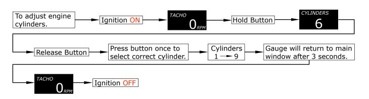
**Installation Tip:** For with vehicles with no tach wire or tach wire location is not know, set cylinder to (1) and connect signal wire (green) to **ONE** cylinder coil only! (e.g. **VE Commodore / FG Falcon)**
