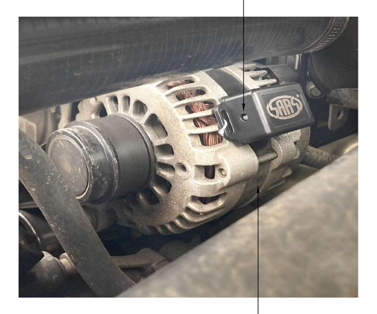
For the best performance, mount tach adapter to the thinnest centre section of the alternator
