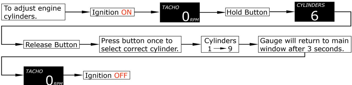
**Installation Tip:** For with vehicles with no tach wire or tach wire location is not know, set cylinder to (1) and connect signal wire (green) to **ONE** cylinder coil only! (e.g. **VE Commodore / FG Falcon**)
