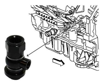
NOTE: Please do not over-tighten the adaptor as this may cause the nylon washer to distort. Doing this could then cause the adaptor to leak.
