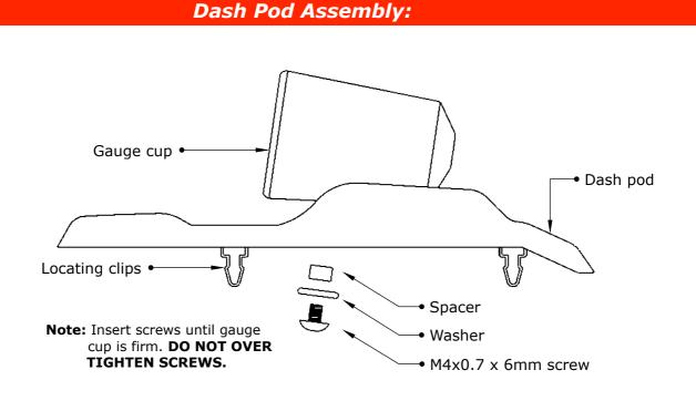
Installing Gauges to Cups:
