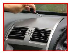
Carefully remove the original cover by prying it open with a flat object (screwdriver or similar). Clips are at the rear.
