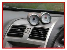
6. Gently and evenly push the new gauge dash pod into position ensuring the clips lock into place.
