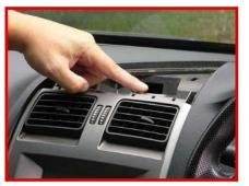
Part of the plastic under the cover needs to be cut away as it interferes with the new gauge pod. While open, proceed to wire the gauges.
