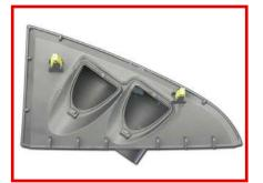
Position clips around the gauge pod ready to mount back in place of the original part.
