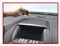
Carefully remove the original cover by prying it open with a flat object (screwdriver or similar). Clips are at the rear.
