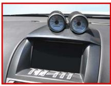
6. Gently and evenly push the new gauge dash pod into position ensuring the clips lock into place.
