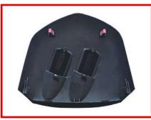
3. Position clips around the gauge pod ready to mount back in place of the original part.
