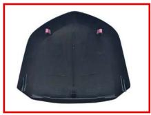
2. Remove the clips from underneath the original cover so they can be attached to the new gauge pod.
