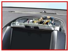
5. While open, proceed to wire the gauges before placing the new gauge pod into position.
