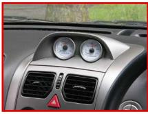
5. Gently and evenly push the new gauge pod into position ensuring clips lock into place.
