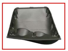
3. Position clips around the gauge pod ready to mount back in place of the original panel.
