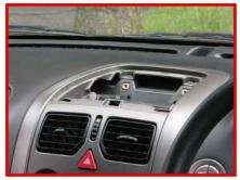
4. While open, proceed to wire the gauges before placing the new gauge pod into position.
