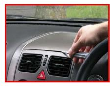
Carefully remove the original cover by prying it open with a flat object (screwdriver or similar). Clips are at the front.
