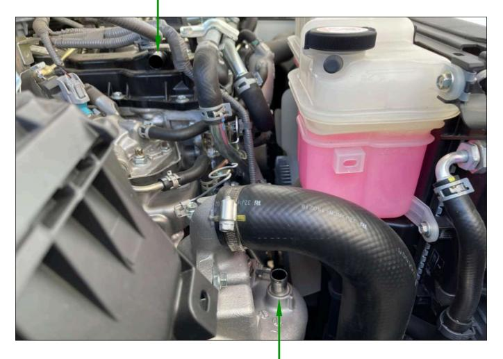
(**OUT**) Hose location from tank to intake (16mm)
