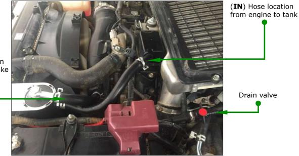
(**OUT**) Hose location from tank to air intake
