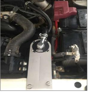
**Step 4:** Fit the tank and bracket to the radiator support using the supplied bolts/washers in the location show above with the drain valve attached to the tank.(Optional)
