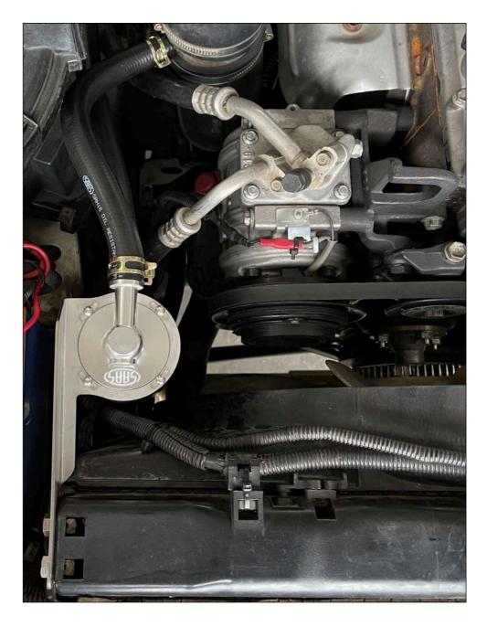
**Step 6:** Cable tie the drain valve in a easy to get to location. (Optional)
