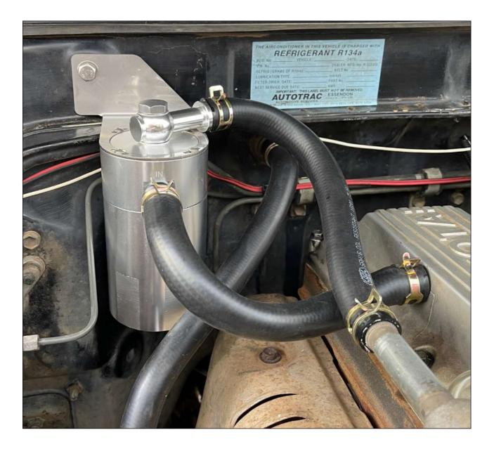
**Step 6:** Cable tie the drain valve in a easy to get to location. (Optional) **Step 7:** Check all work before starting engine.
