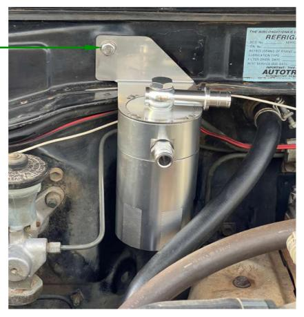
Remove factory bolt from firewall and replace with supplied bolt /washer
