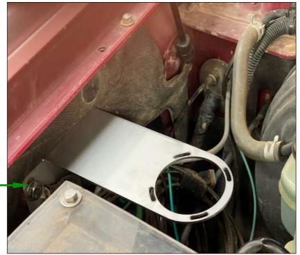
Use the supplied M8 bolts and washers to mount bracket in location shown
