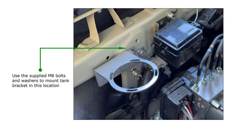
Step 3: Fit tank to bracket. If you wish to use the supplied drain valve, attach the drain valve before mounting the tank to the bracket.
