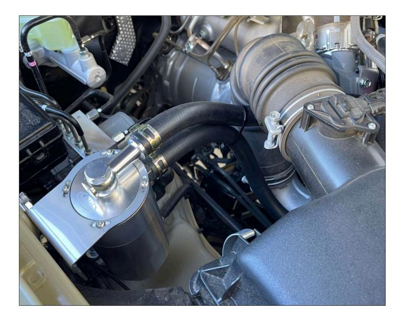
**NOTE:** SAAS recommends checking your catch tank after traveling 1000km, to see how much oil has accumulated in the tank. It is important that the build-up of oil does not rise above the internal baffle, through to the bronze filter.
