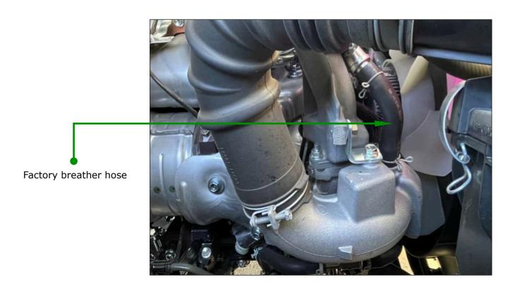
**Step 5:** Connect (**IN**) hose from engine to tank. See page 5 for layout. **Step 6:** Connect (**OUT**) hose from intake to tank. See page 5 for layout.
