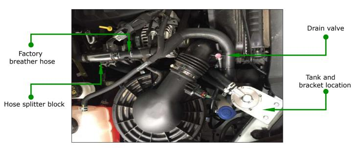
**Step 8:** Cable tie the drain valve in a easy to get to location. (Optional) **Step 9:** Check all work before starting engine.
