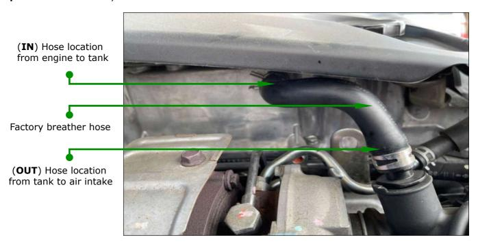
**Step 3:** Fit tank and bracket in location shown below with the drain valve attached to the tank.(Optional)
