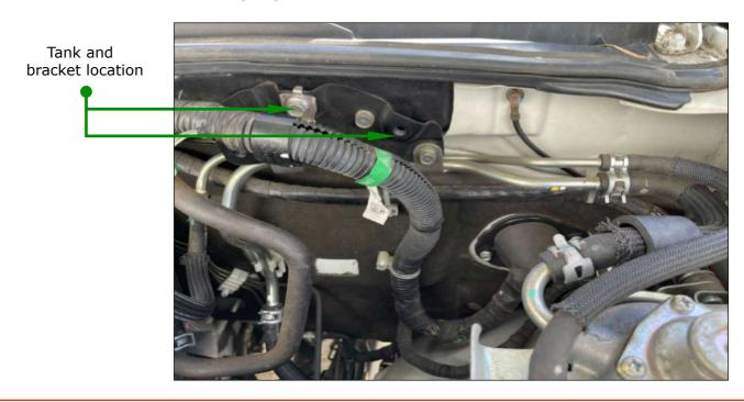
**NOTE:** SAAS recommends checking your catch tank after traveling 1000km to see how much oil has accumulated in the tank. It is important that the build-up of oil does not rise above the internal baffle through to the bronze filter.
