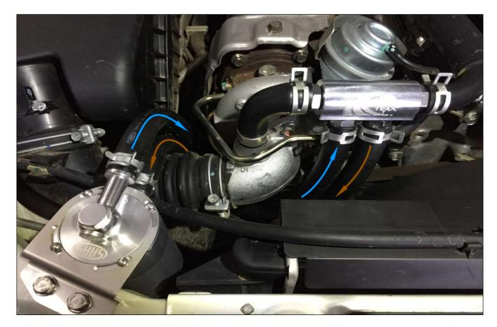
**Step 7:** Cable tie the drain valve in a easy to get to location as shown below. (Optional) **Step 8:** Check all work before starting engine.
