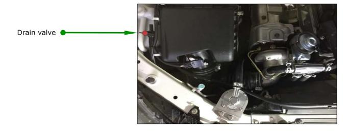
**NOTE:** SAAS recommends checking your catch tank after traveling 1000km to see how much oil has accumulated in the tank. It is important that the build-up of oil does not rise above the internal baffle through to the bronze filter.
