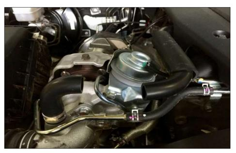
**Step 4:** Fit the hose splitter block to the factory breather hose shown below. Use the 2 larger hose clamps supplied.
