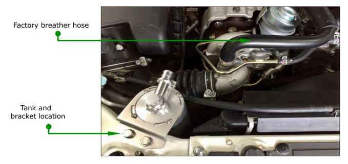
**Step 3:** Cut out a 75mm section from the factory breather hose shown below.
