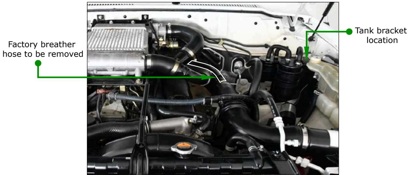
**Step 5:** Connect (**IN**) hose from engine to tank in location shown below.(See page 3 for layout)
