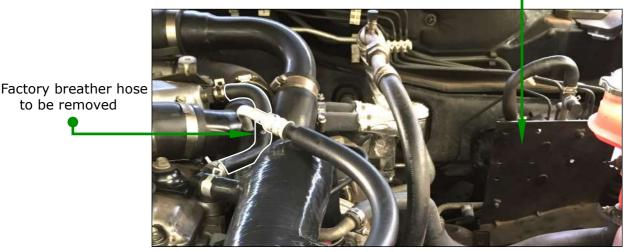
Step 5: Connect (IN) hose from engine to tank in location shown.
