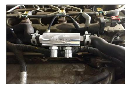
**Step 6:** Fit tank and bracket using the supplied blots/washers in the location shown below with the drain valve attached to the bottom of the tank.
