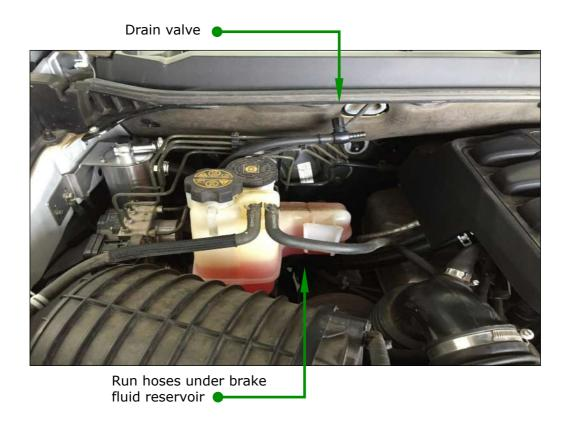
**NOTE:** SAAS recommends checking your catch tank after traveling 1000km to see how much oil has accumulated in the tank. It is important that the build-up of oil does not rise above the internal baffle through to the bronze filter.
