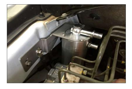
**Step 7:** Connect (**IN**) hose from engine to tank through hose splitter block. (See page 4 for layout)
